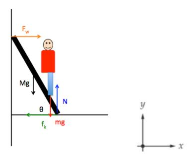
We need to find  $f_k$ . Other unknowns are the normal force N and the wall force  $F_w$ . We have three unknowns and three equations (translational equilibrium along x and y and rotational equilibrium). We choose the point at which the ladder touches the floor as axis of rotation.
