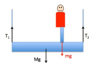
We can solve the problem imposing that the net-torque acting on the scaffold+man system is =0:
