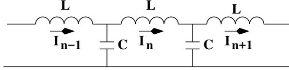
Figure 1: An infinitesimal element of a delay line
