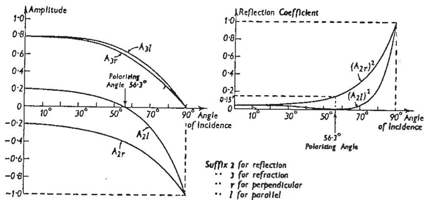
Fig. 21-3. Reflected and refracted amplitudes for  $n'/n=1.5$ .
