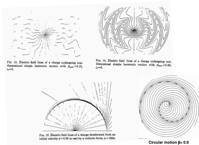
Figure 2: Examples of the electric field for an accelerated charge
