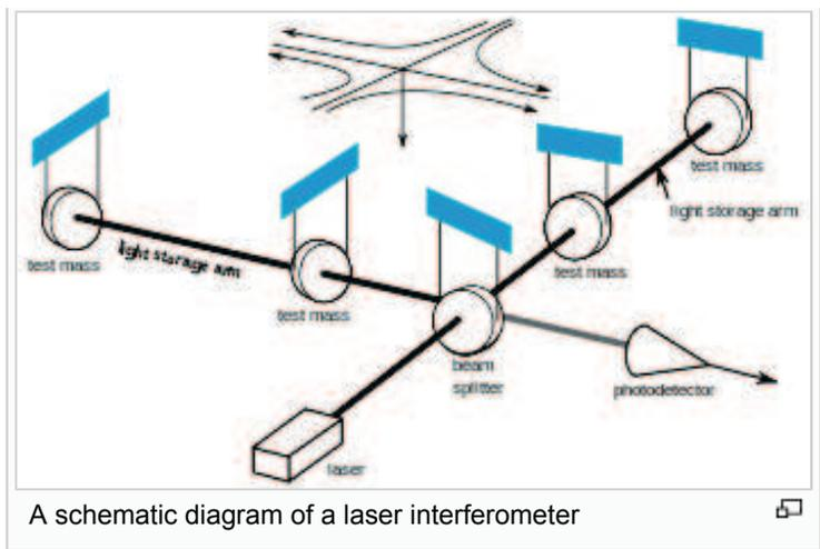
Figure 3: A sketch of a laser interferometer system such as employed by LIGO
