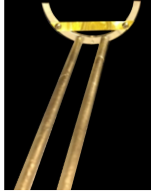
Figure 22: Fixed target apparatus including support beams, holding collar and gold foil. Figure from [39].
