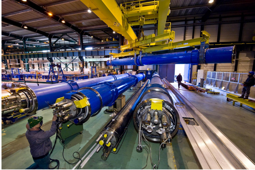
Figure 2.11: The cryodipole magnets testing before the installation at LHC
