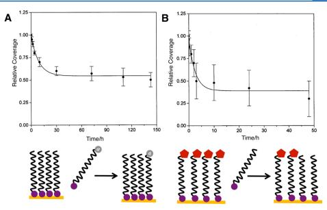
**Figure 4.** Relative coverage of (A)  $CH_3(CH_2)_{19}SH$  in a SAM dipped in a  $CD_3(CH_2)_{19}SH$  solution and (B) ferrocene-terminated thiols in a SAM dipped in  $CH_3(CH_2)_{11}SH$  solution over time. Adapted with permission from ref 57. Copyright Elsevier 1999.
