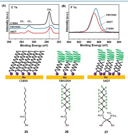
**Figure 12.** Homogeneously mixed multicomponent spiro adsorbates for exploring the interfacial properties of surfaces containing well-defined mixtures of hydrocarbons and fluorocarbons. Results of XPS analysis of (A) C 1s and (B) F 1s binding energy regions of normal alkanethiol, partially fluorinated spiroalkanedithiol, and partial fluorinated SAMs. Reproduced with permission from ref 121. Copyright 2015 American Chemical Society.
