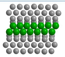
**Figure 2.** Illustration of a mixed SAM as viewed from above showing how adsorbates with two dissimilar chains avoid the formation of large domains. (Terminally fluorinated chains are represented by filled green circles.) Reproduced with permission from ref 29. Copyright 2012 American Chemical Society.
