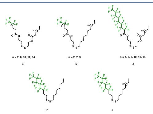
Figure 7. Structures of fluorinated disulfide adsorbates used for fundamental studies in the generation of mixed monolayer films.<sup>32,76</sup>
