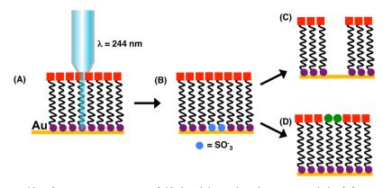
**Figure 8.** Patterning SAMs on gold surfaces using scanning near-field photolithography. This process includes (A) scanning the SAM using UV light, (B) photochemical oxidation of exposed thiolates to sulfonates, (C) selective etching of gold surfaces, and (D) displacement of the oxidized adsorbate molecule. Reproduced with permission from ref 82. Copyright American Chemical Society 2002.
