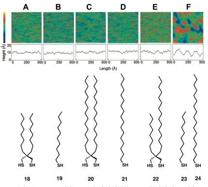
**Figure 11.** AFM images (topographic) of SADT SAMs (A)  $C10C10(SH)_2$  (**18**), (C)  $C17C17(SH)_2$  (**20**), and (E)  $C10C17(SH)_2$  (**22**) along with normal alkanethiols (B) C10SH (**19**), (D) C17SH (**21**), and (F) a mixed SAM where [C10SH]/[C17SH] = 2. Reproduced with permission from ref 120. Copyright 2000 American Chemical Society.
